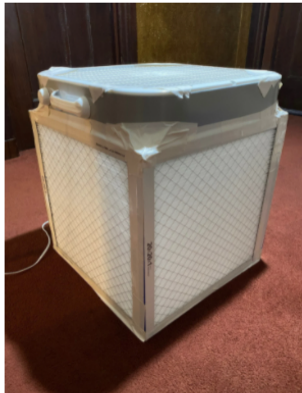
Figure 1. A Corsi-Rosenthal Cube. This cube was constructed with 4 MERV-13 filters and features a cardboard bottom.
