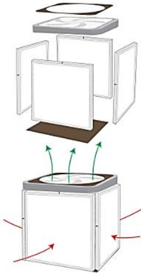
Figure 2. A visual guide to constructing a Corsi-Rosenthal cube with a box fan and MERV filters with a top fan configuration. Air is pulled into filters (red arrows) and blows out of fan (green arrows). Photo by CC-BY al.hu .
